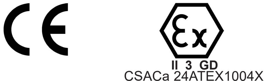
Figure 1. Markings on the Front of Sensor
