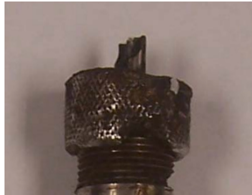
remnants of a CTC A2A connector where the polycarbonate has completely disintegrated and the stainless locking ring has been seriously eroded due to the sulfuric acid
