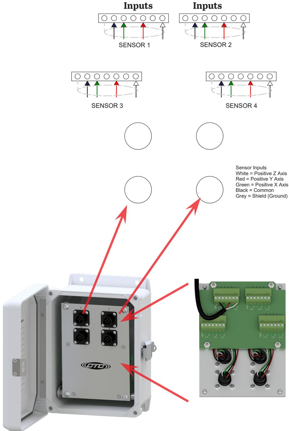
**Figure 10. Field Wiring for 4-Conductor Triaxial Sensor Inputs**
