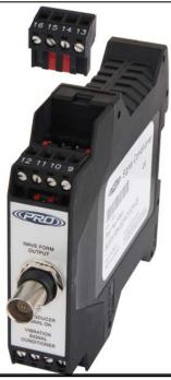
SC200 series Signal Conditioner. Provides 4-20 mA and 0-5 V or 0-10 V outputs proportional to vibration turned off. This is done on one of the two pages in RBM Ware, during measurement point setup.
