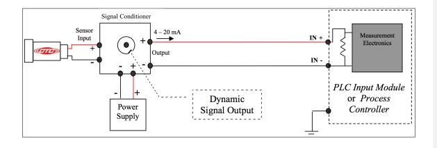
The four wires needed to monitor overall vibration level using a signal conditioner are:
