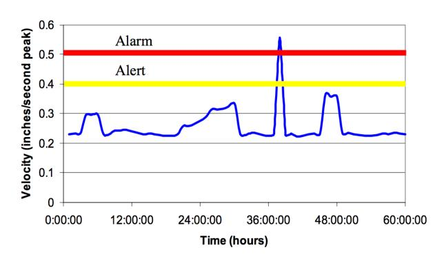
Example of a loop power sensor's output vs. time
