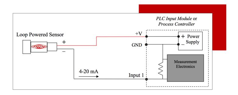
The sensor can be wired directly into analog input modules on PLCs or Process Controllers that accept 4-20 mA signals
