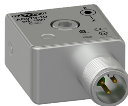
AC979 Nonincendive, intrinsically safe, X and Z axes, 100 mV/g, ±10% sensitivity tolerance
