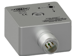
TXFA331-VT Premium, piezo velocity and temperature output, 500 mV/in/sec, 10 mV/°C, ±5% sensitivity tolerance
