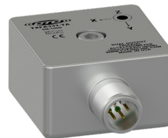
TXFA331-TA Premium, acceleration and temperature output, 500 mV/g, 10 mV/°C, ±5% sensitivity tolerance
