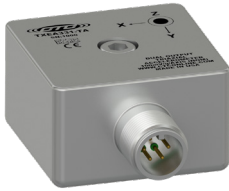
TXEA331-TA Premium, acceleration and temperature output, 100 mV/g, 10 mV/°C, ±5% sensitivity tolerance
