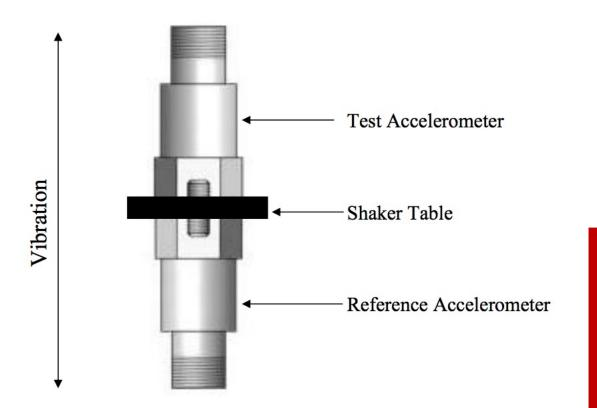
Stud mounting is accomplished with a drilled and tapped hole using a threaded fastener between the accelerometer and the machine.
