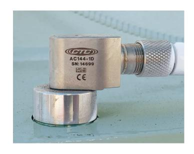
Under ideal circumstances, the accelerometer mounting method should provide total use of the transmission region.
