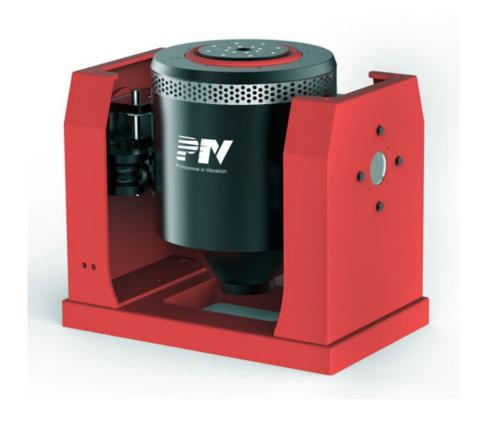
A vibration shaker with a calibrated standard reference accelerometer built into it will be used to simulate the machine vibration.
